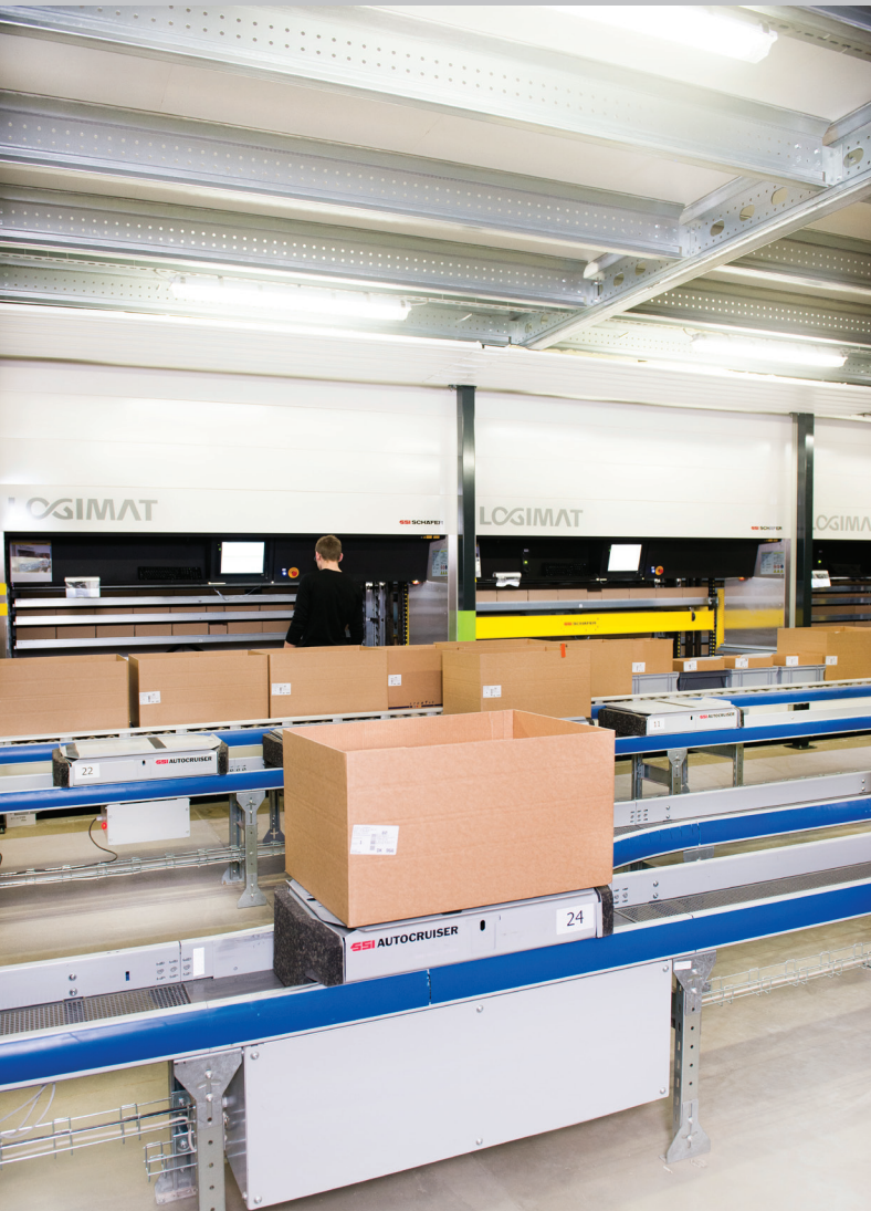
Unique combination of transport system and vertical lift
