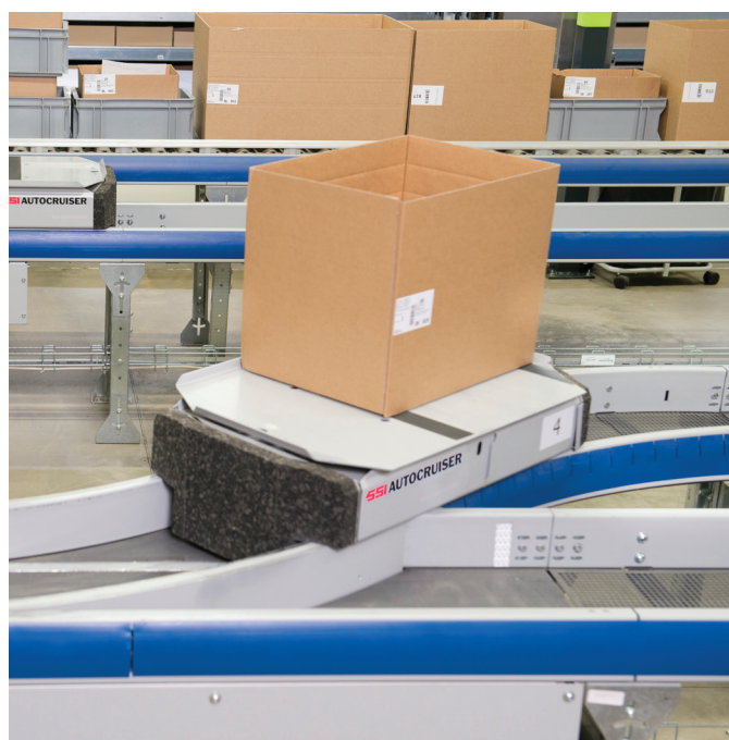
27 SSI Autocruisers on a 300 m long track
